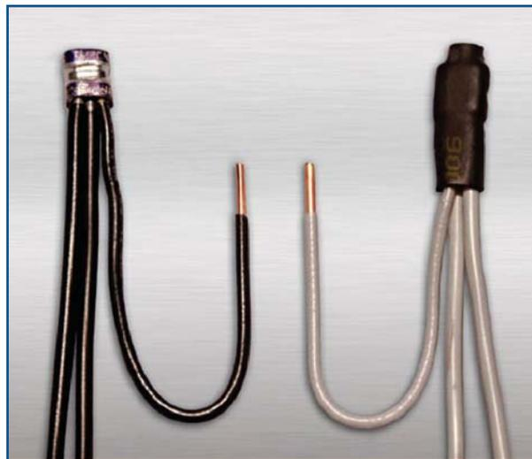
The tool is shown in the illustration below. An insulating sleeve is placed around the crimp connector to complete the repair. The copper wire pigtail is then connected to the switch, receptacle, or other termination device. An example of a repaired receptacle outlet is also illustrated below.
